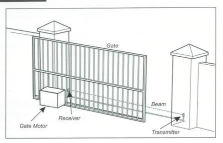
The above drawing shows a standard application of the *wireless* INFRA-RED beam, in use as a safety beam for a sliding gate. The transmitter and receiver pair are mounted a distance above the ground (typically 30cm) and in such a manner that they are facing each other and are aligned i.e. the beam travels in a straight line. To aid alignment, the receiver has a LED on the board, which will illuminate if the transmitter's signal is received.
